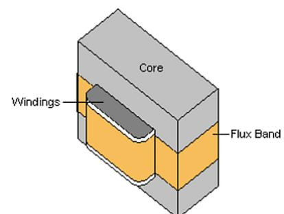
our DIY Faraday Cage design is to put a continuous sheet of highly conductive material around the entire body of the DIY Faraday Cage, so that AM radio signals, and other lower frequency EM sources (such as 'Dirty Power') are attenuated or eliminated by the current flowing in that 'Flux Band.'
