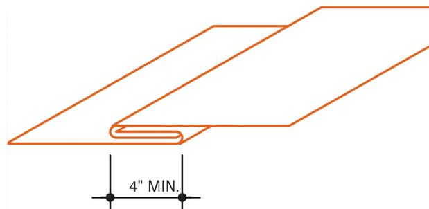
The copper mesh loop can be cut if absolutely necessary, with a seam like this held under pressure between two timber or metal spars. This construction was used in the whole-bedroom Faraday Cage shown above.
